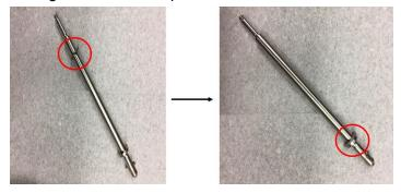
2. Place cylindrical metallic piece on the end of the inner tool piece:
