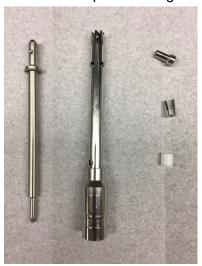
1. Make sure plastic o-ring is on inner tool piece:
