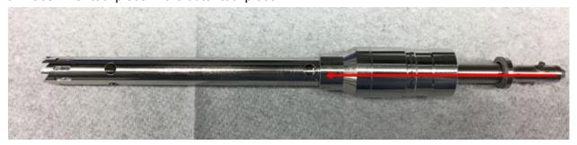
4. Place the large plastic bushing piece in the sharp end of the outer tool piece, and then the metallic rotor:
