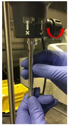
8. The homogenizer is now setup to run.
