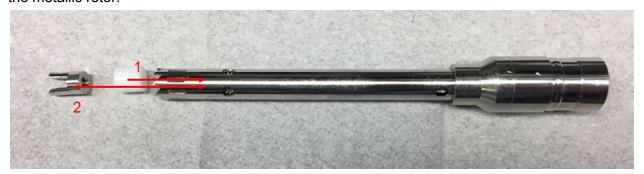
5. Screw in the rotor using the screw pieces. Don't overscrew the rotor in! Only turn the pieces until the rotor is tight. Hold the left piece and rotate the right handle clockwise to tighten:
