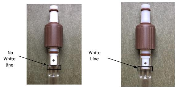
We've had a problem with over-tightening the Teflon screw valves. You can tell if a Teflon valve has been over tightened by the shape of the hole at the bottom of the valve - if it's a circle, it's fine to use. If it's an oval, it's been crushed through over tightening at some point in the past, and may not seal the tube as well.
