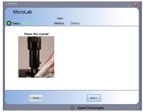
Any solvent may be used for cleaning the ATR, since the window is made of diamond (therefore, it is chemically resistant). The DialPath has less chemical resistance (because its window is made of ZnSe), therefore, only use solvents that are compatible with ZnSe optics.
