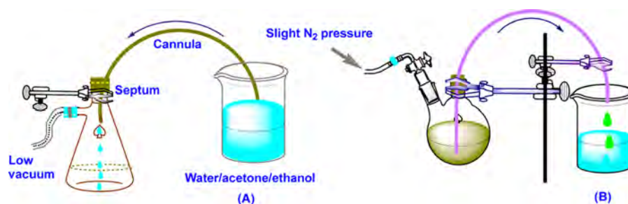
Figure 9. Cleaning cannulas using a vacuum (A) or nitrogen (B).
