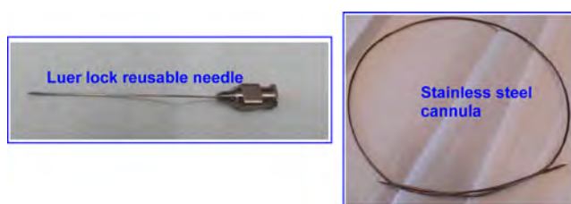
Figure 4. Needles and cannulas used in chemistry laboratories.
